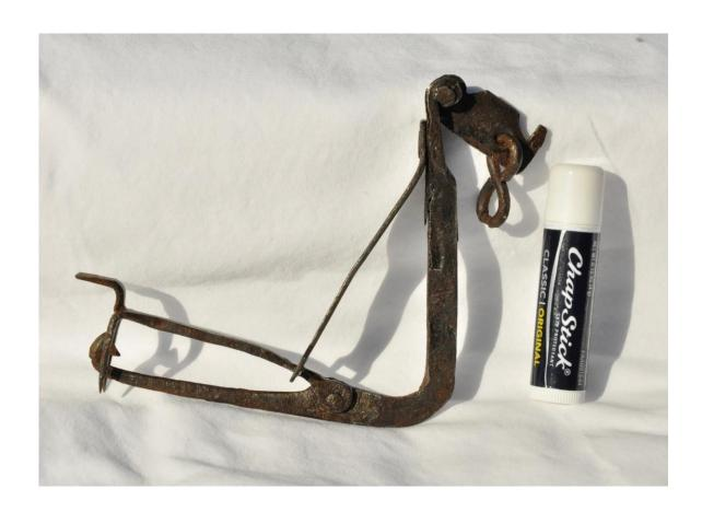
To set the trap as shown below, the spring is first compressed, which allows the striking arm to rotate upon its pin, so that the L-shaped extension opposite the dual spikes is able to latch into the notch on the piece attached to the S-shaped line-tie, which spins around its own pin and serves as the "dog" of this trap.
