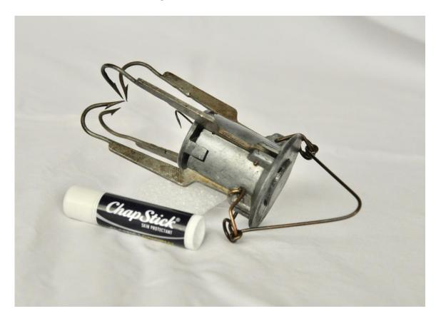
The Payne Trap as seen from underneath. Note the circular plate through which the bait is attached which springs the trap shut when pushed upward.
