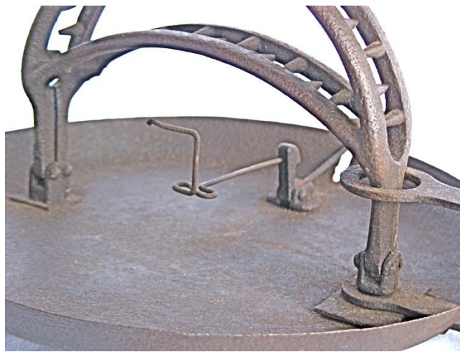
Figure 1c. Close-up of the Evans' Fryin' Pan Trap Setting Mechanism
