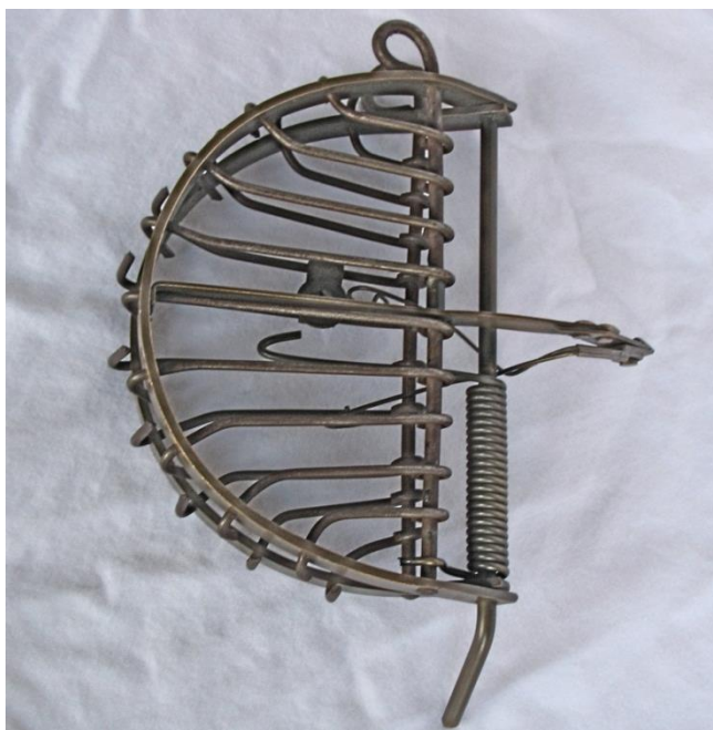
Figure 5a. Turner and Fletcher Fish Trap in the Closed ( Sprung ) Position
