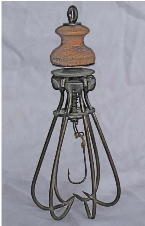
Figure 4a. Lake Erie Claw Trap in the Sprung Position
